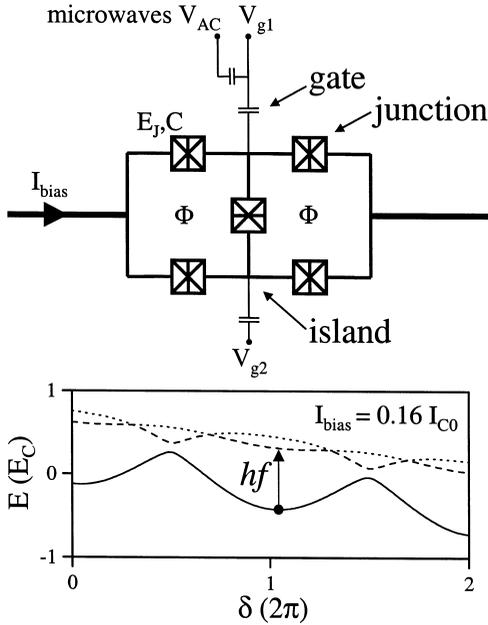
Fig. 1. Top: Schematic of the array. Here we only consider the case of symmetrically induced gate charges for the top and bottom island  $n_g = C_g V_g / 2e$ , and a magnetic flux  $\Phi = 0$  applied to the loops. Bottom: The lowest three bands of the array as a function of the phase  $\delta$  across the array, here calculated for  $E_J/E_C = 0.3$  and  $n_g = 0.37$  using [6]. At finite bias current the bands are tilted ( $I_{C0} = (2e/\hbar)E_J$ ).
