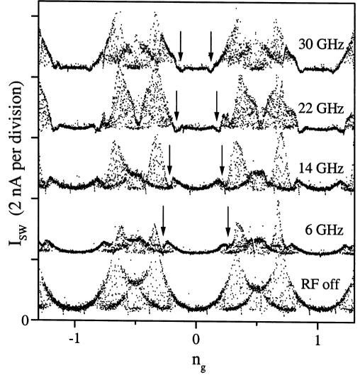
Fig. 2. Measurements of the  $2e$ -periodic modulation of the switching current  $I_{SW}$  by the dimensionless gate charge  $n_g$ , measured with different microwave frequencies, at a temperature of 10 mK. Data sets are 2 nA offset for clarity.
