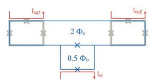
permanent magnet. The current response to a flux change is very small. In the on state, the flux in the SQUID loop is made integer by means of a control current  $I_{ct}$  (red). As the transporter attempts to keep the flux in its loop constant, a flux change induced by qubit 1 is transmitted to qubit 2. As shown here, the two three-junction qubits experience  $\sigma_z \otimes \sigma_z$ -type coupling. The flux values have to be adjusted for the influence of circulating currents.
