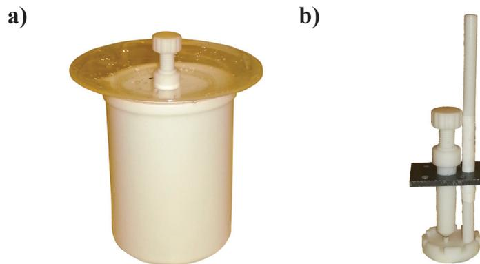
**Figure B.1:** **a**, Custom made tool for suspended submission of GaAs into hydrofluoric acid. The teflon pen is put through a hole in a polyethylene dish. **b**, Custom made tool for the drying step with the GaAs epilayer on Sapphire. Contact between sapphire and the GaAs epilayer is made under water, to prevent dust particles at the interface of GaAs and sapphire.
