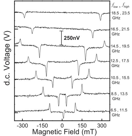
FIG. 2. The dc voltage  $\Delta V$  generated by a Pt/Py/Al device in response to the rf magnetic field plotted as a function of the static magnetic field. The frequencies of the rf field are as shown. The peaks (dips) correspond to resonance at  $f_{\text{high}}$  ( $f_{\text{low}}$ ). The data are offset vertically, for clarity.
