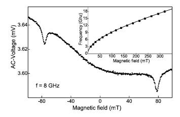
FIG. 2. Measured ac voltage as a function of static magnetic field for an applied rf magnetic field at frequency of 8 GHz. The inset shows the static magnetic field dependence of the resonance frequency, as derived from the dips in the ac voltage vs magnetic field. The squares represent the experimental data, the curve is a fit to the data; using the Kittel formula.
