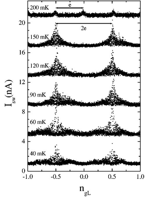
FIG. 2. Switching-current results (dots) versus  $n_{gL}$  for different temperatures,  $n_{gR} = 1/2$  and  $\Phi = 0$ . The curves are offset  $4 \text{ nA}$  for clarity. The odd-even transition temperature was  $190 \text{ mK}$ , while the main peaks partly collapse below  $\sim 80 \text{ mK}$  due to poisoning effects (see text).
