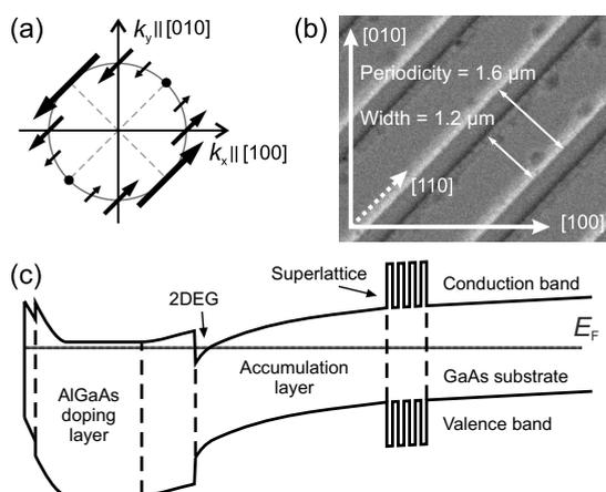
FIG. 1. (a) Dependence of spin-orbit fields on  $k$  vector on the Fermi circle in the  $k_x$ - $k_y$  plane for equal strength of Rashba and linear Dresselhaus effect. (b) Scanning-electron micrograph for a section of a wire array oriented along the [110] crystal direction. (c) Band diagram of the GaAs/AlGaAs heterostructure (not to scale), with a 2DEG where the conduction band bends below the Fermi energy  $E_F$ .
