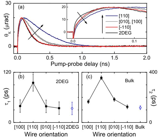
FIG. 2. (Color online) Spin-dephasing anisotropy at zero external magnetic field. (a) Kerr rotation as a function of pump-probe delay for the unpatterned area and wires in  $[-110]$ ,  $[110]$ ,  $[100]$ , and  $[010]$  directions (order along arrow in traces and legend match). The inset shows the Kerr response at short delays to highlight the slow growth in all traces. [(b) and (c)] Spin-dephasing times for both the 2DEG ( $\tau_1$ ) and bulk ( $\tau_2$ ) spin populations.
