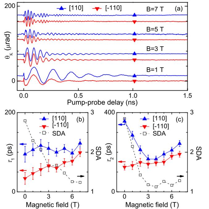
FIG. 3. (Color online) Evolution of SDA in transverse magnetic fields up to  $B=7$  T. (a) Kerr signals as a function of pump-probe delay from  $[110]$  and  $[-110]$  oriented wires (traces offset for clarity). [(b) and (c)] Corresponding spin-dephasing times  $\tau_i$  as a function of  $B$ , for (b) 2DEG and (c) bulk electrons. These plots also present SDA quantified as  $\tau_{i,[110]}/\tau_{i,[-110]}$ .
